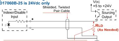
RLD may be needed in applications using a PLC DC output to generate index pulses at high speeds. See the note on this page for more information.
