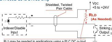
RLD may be needed in applications using a PLC DC output to generate index pulses at high speeds. See the note on this page for more information.
