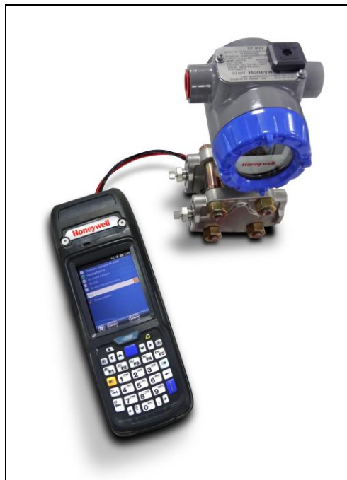
Figure 3-3 Connecting to a device through MCT404
