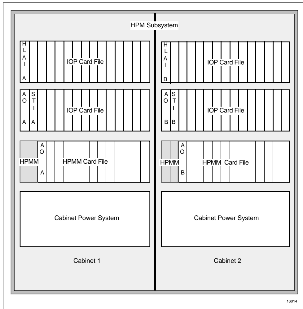
Figure 10-2 Dual Cabinets with Redundant HPMMs
