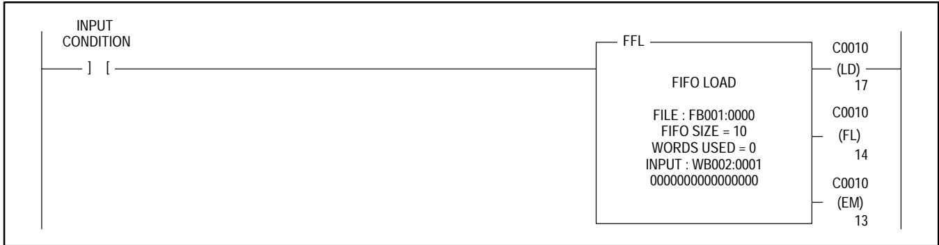
Figure 9.8 Example Rung for a FIFO-load Instruction
