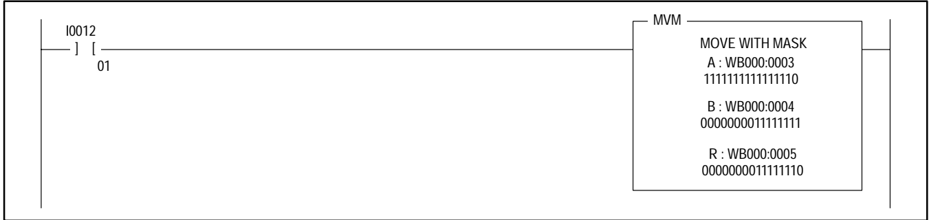
Figure 6.4 Example Rung for a Move-with-mask Instruction
