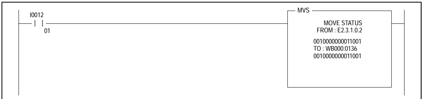
Figure 6.5 Example Rung for a Move-status Instruction
