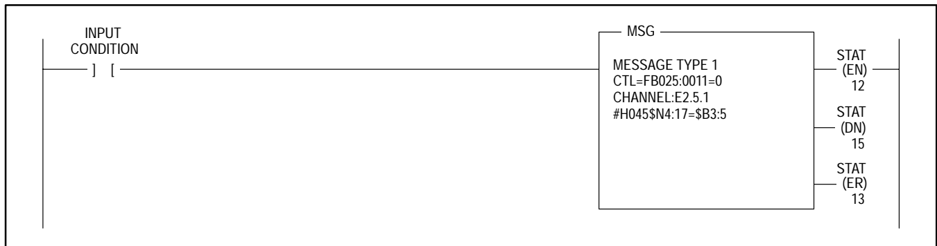
Figure 16.6 Example Rung that Executes a Data Highway Command on a Communication Adapter Module
