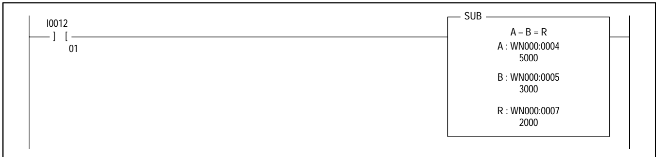
Figure 6.14 Example Rung for a Subtract Instruction
