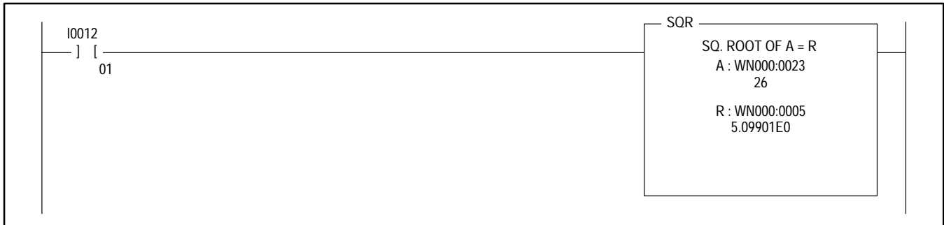
Figure 6.17 Example Rung for a Square-root Instruction
