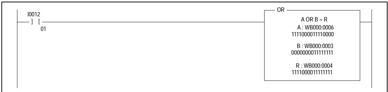
Figure 6.20 Example Rung for an OR Instruction
