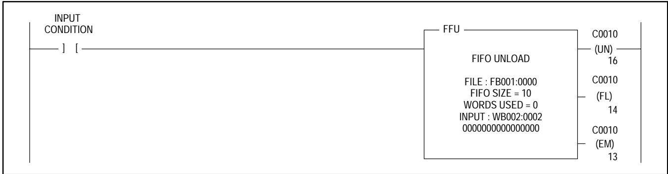
Figure 9.9 Example Rung for a FIFO-unload Instruction
