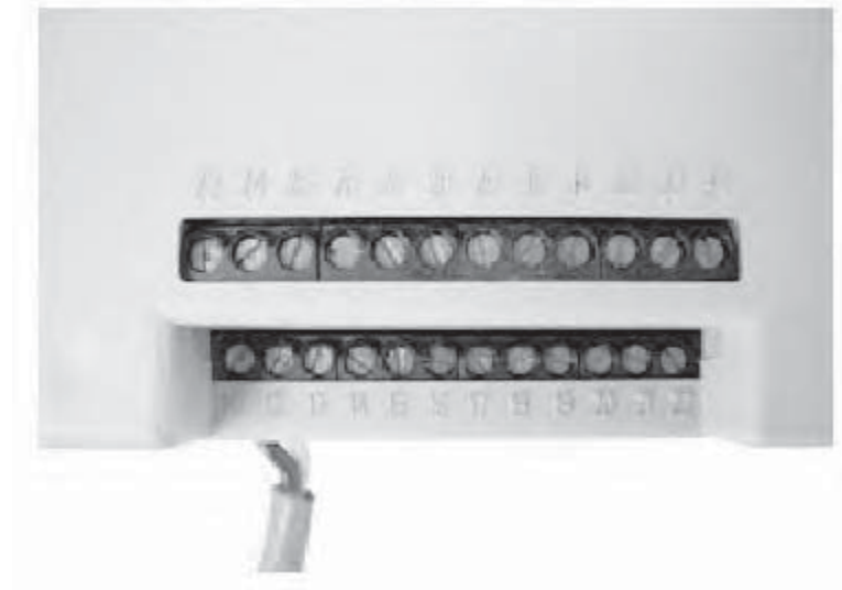
Figure 2.10 – SMC-Flex Controller Control Terminals
